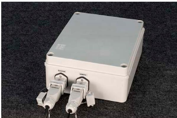
Fig.6-2 - Connettori Azimuth - Elevation
